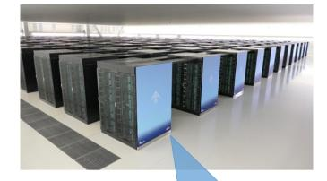
Fujitsu Supercomputer Fugaku New TOP500 1<sup>st</sup> place 22/06/20 158K+ nodes based on 48-core A64FX ARM SoC
