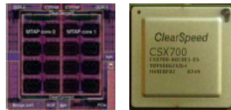
Figure 1: The CSX700 192-core embedded processor
