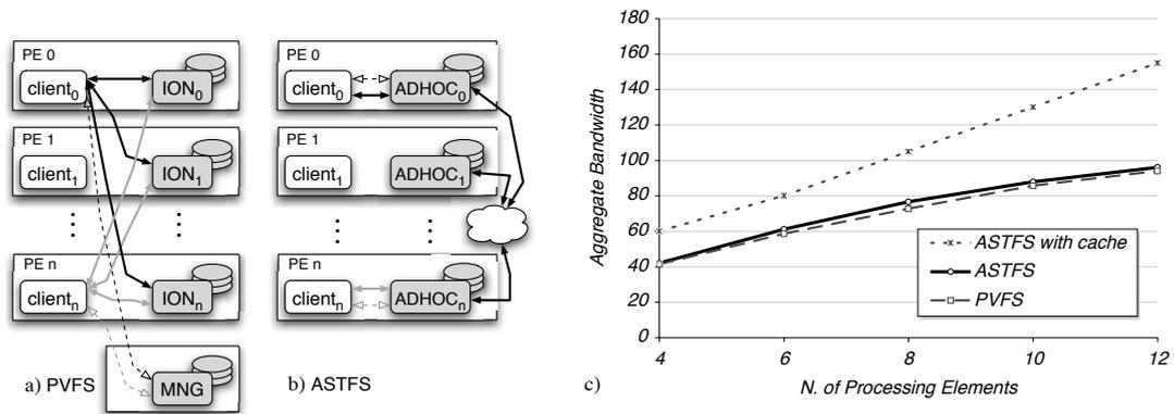
Figure 5. a) Many clients accessing a PVFS. Each PE hosts a client is required to be an ION. Solid edges show data paths, dashed edges meta-data paths. b) Many clients accessing an ASTFS. c) Comparison among PVFS and ASTFS. Each client read a partition of the file in segments of 10MB randomly chosen within its partition. In both cases, each client reads the same 800MByte file spread among all PEs.
