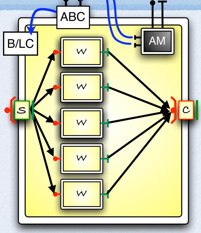
ABC = Autonomic Behaviour Controller (implements mechanisms)AM = Autonomic Manager (implements policies)B/LC = Binding + Lifecycle Controller13
