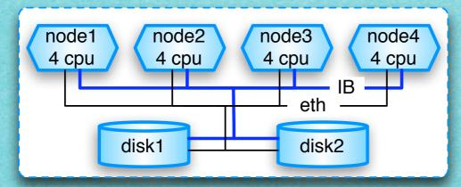
Physical Cluster + external SAN InfiniBand + Ethernet 4 Nodes x 4 CPUs Cluster InfiniBand 192.0.0.0/24 Cluster Ethernet 192.0.1.0/24 Internet Gateway 131.1.7.6
